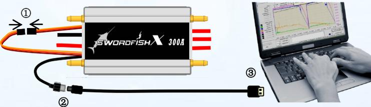
Step ①: Short upgrade cable with receiver wire.
