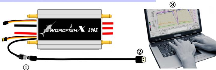
Step ①: Correctly connect ESC's Wifi wire/to USB adaptor wire to USB adaptor
