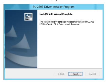
4. Plug in the USB to Serial adapter to the PC USB port. Windows should detect the driver as "Prolific USB-to-Serial Comm Port". Go to Device Manager and check for the device and the COM port number assigned by Windows. You can also check the driver version by right-clicking on the "Prolific USB-to-Serial Comm Port" device and select Properties and Driver tab.
