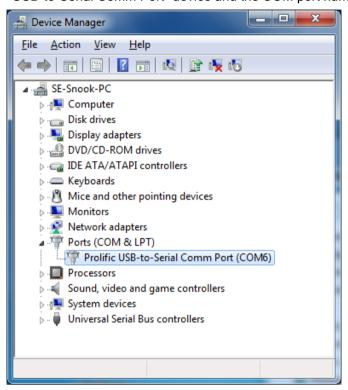
You can also check the driver version by right-clicking on the "Prolific USB-to-Serial Comm Port" device and select Properties and Driver tab.
