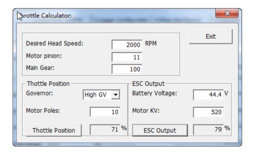
Incorrect gear rate/motor KV probably results the ESC Output haven't enough reserve to compensate battery voltage decreasing and load change, in the case there is a tab pop out to indicate 'Head Speed Out of Control Range'. Generally you can Inc/Dec the tooth of motor pinion or Inc/Dec the Desired Head Speed to get the best match results. Please carefully check your heli configuration, make sure the desired heed speed is under control
