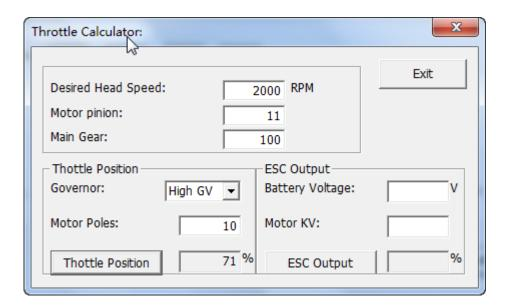
Furthermore, fill out the battery voltage and motor KV can help you find out the ESC power output match with the pre-set head speed, HiFei recommends for optimum the ESC output to motor about 80% power, it ensure the ESC has enough reserve to compensate the battery voltage decreasing and load changing. Please see the following screenshot:
